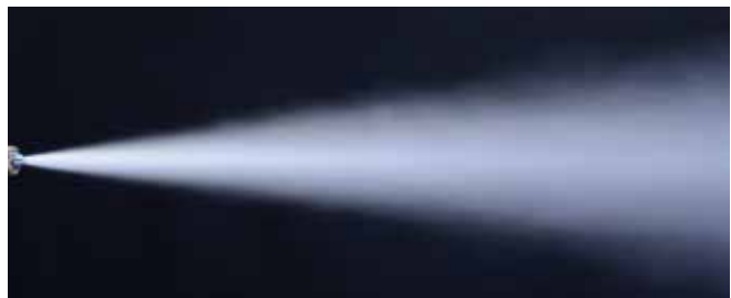
Spray pattern of a Laval nozzle
