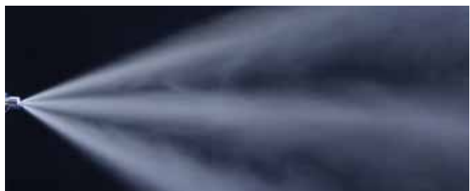
Spray pattern of the flat fan nozzle
