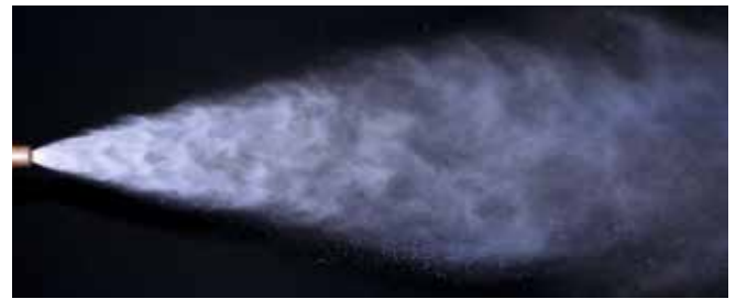
Spray pattern of the MasterNOx® nozzle 30°
